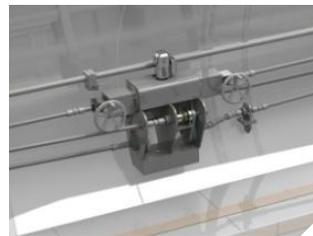
*A single motor fulfils all of the functions: unlocking, balancing of pressure, rising/lowering of the door, rotation. As well as saving space, this single block simplifies the electrical control, reduces the number of mechanical components and increases the security of the interlocking of doors.*
